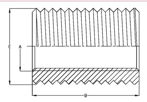
Female thread A = M8Length B= 12Male thread E= M12Type= 97x 000 080.120
